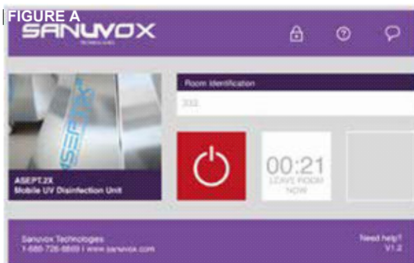
The pre-timer “countdown operation” gives the user 30 seconds to leave the room prior to the ASEPT.2X activating.
