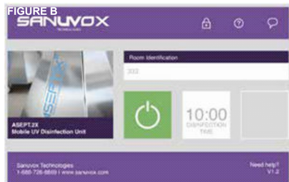
The pre-timer “countdown operation” gives the user 30 seconds to leave the room prior to the ASEPT.2X activating.
