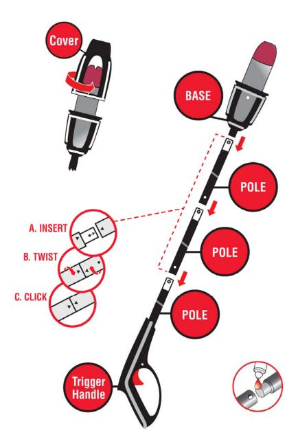
(Assembly Tip: To make assembly easier, add a small drop of liquid soap at the tip of the connector, then insert and twist! To improve grip during assembly, use rubber gloves.)
