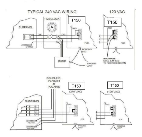
Note: Wire the pump directly to the time clock—do not use the THANOS T150 as a junction box.
