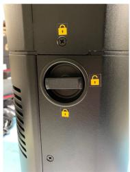
d. Turn the latches on both sides of the unit to align with the upper and lower lock symbols.
