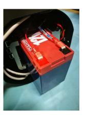
e. Disconnect the positive (red) and negative (black) leads from the battery terminals.
