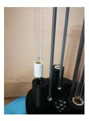
d. Slide the replacement lamp through the top bracket.
