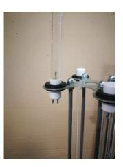
e. The white lines on the side of the lamps should face inwards. This will ensure the lamp pins and the connector key are aligned. Apply gentle downward pressure on the lamp to ensure it is fully seated into the connector.
