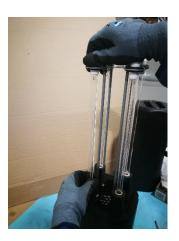
c. Hold the lamp as close as possible to the base of the unit until the lamp is detached from the connector.
