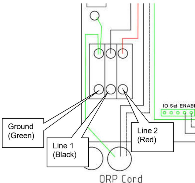
Connect the external control cord to a chemical feed controller or for manual operation, to a 120 volt AC outlet. When connecting to a chemical feed controller, be sure the controller is set to continuous feed and not set on proportional control. Proportional control will reduce the life of power supply components.
