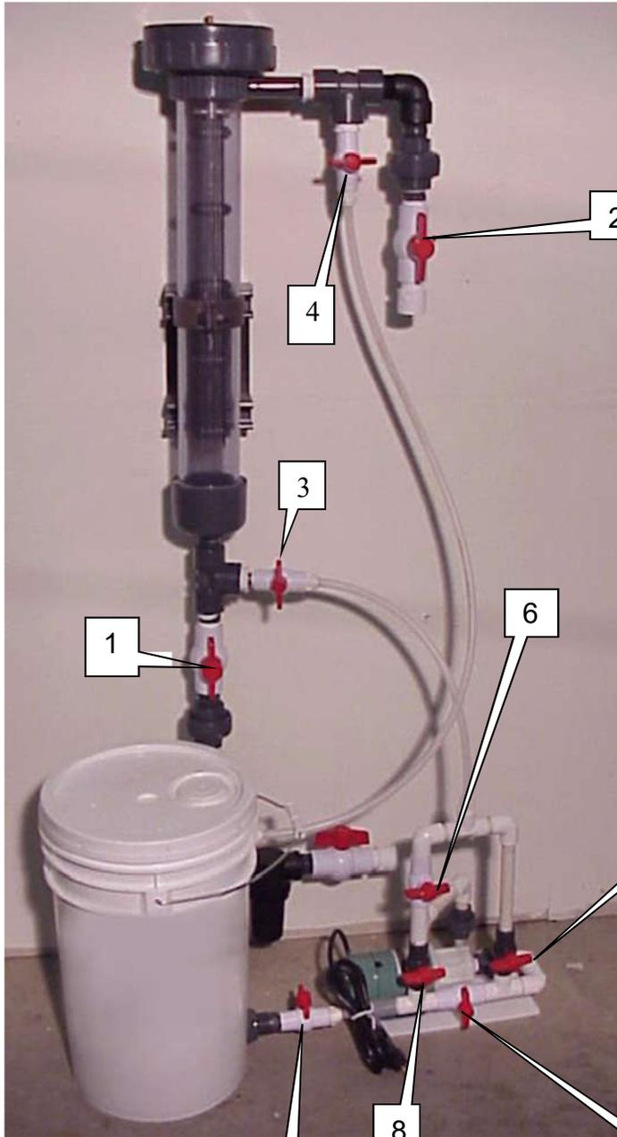
Close all acid wash valves (3), (4), (5), (6), (7), (8) and (9). Open the 2 cell tube valves (1) and (2).
