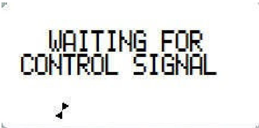
The screen below is displayed when the system detects no flow through the electrolytic cell housing. This condition will stop the system from generating chlorine. Once flow is restored, the system will start automatically and this screen will no longer be active.
