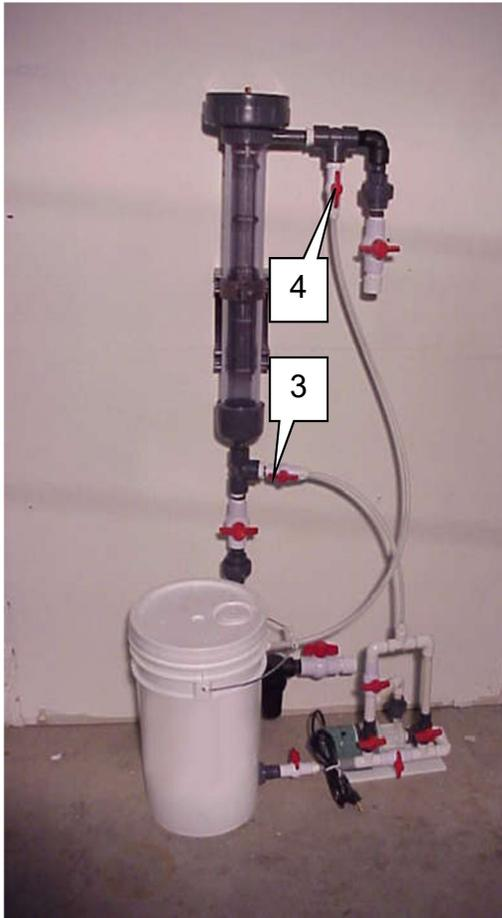
Connect the acid wash tank and pump to the acid wash valves (3) and (4) as shown in the photo.
