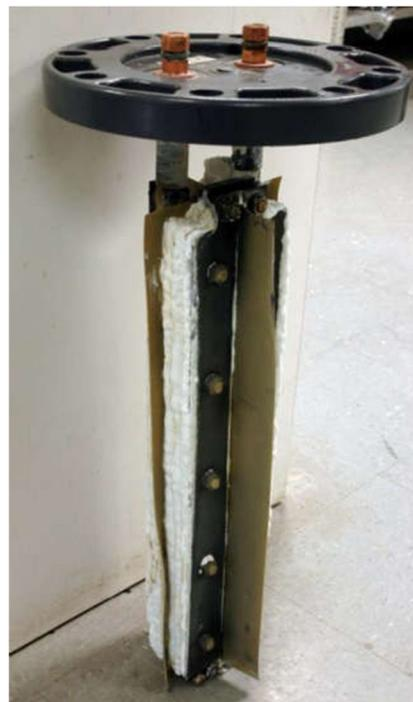
A cell stack with calcium bridged plates.
