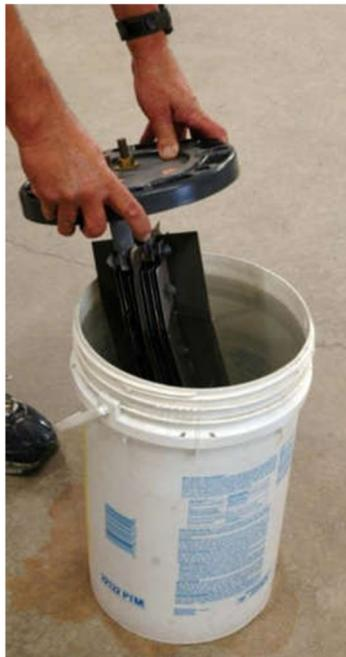
8. Reassemble the cell stack in the tube and reconnect the cables to the top of the cell stack.
