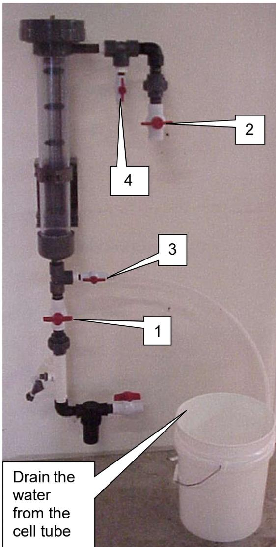
Close the lower and upper cell tube ball valves (1) and (2).
