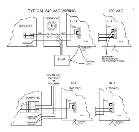
Note: Wire the pump directly to the time clock—do not use the BLH as a junction box.
