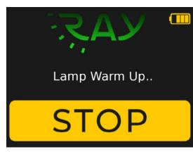
When the lamp warm-up is complete (default warm-up time is 2 minutes), the treatment will commence. The lamps will be fully illuminated and Aero HygenX RAY – Autonomous UVC Robot will start moving down the aisle. (If Aero HygenX RAY – Autonomous UVC Robot has been used in the previous 5 minutes, lamp warm-up reverts to just 30 seconds.)
