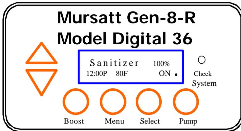
The **MENU Button** allows you to enter the programming and monitoring functions.
