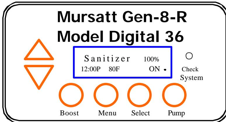
The **SANITIZING OUTPUT LEVEL** is adjustable from 0% (OFF) to 100 % (MAX) by pressing the **Up/Down** Arrows to obtain the desired Sanitizer Output Level. Little adjustment is needed once the initial setting is established.
