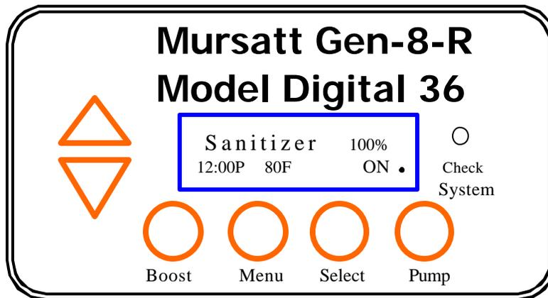
Use **UP/DOWN ARROW** and **SELECT** to scroll through the sub-menu. After completing a step, it displays the next step:
