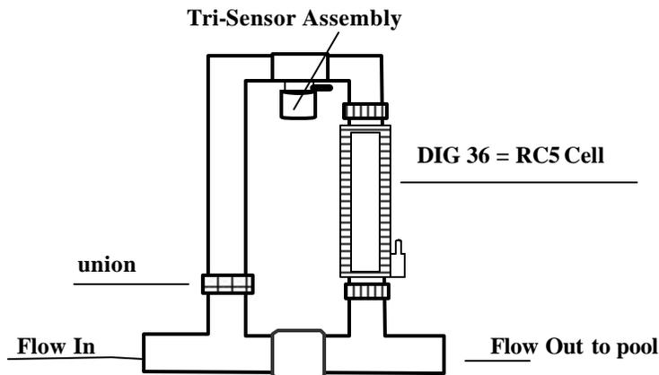
Flow Bypass Manifold Assembly
