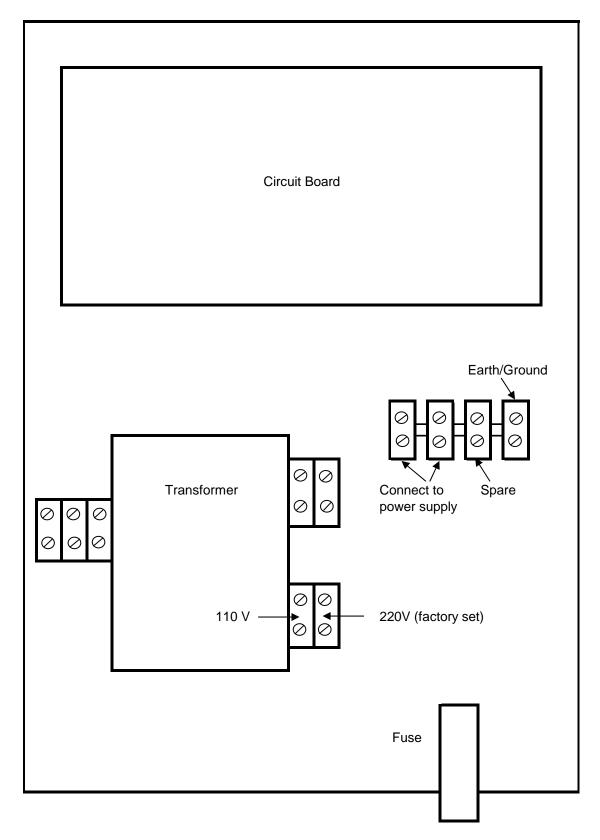
Please note: Power pack must be wired to pump switch terminals. This unit is factory set to be wired to 220V but can be converted to 110V. See inside chassis for directions.
