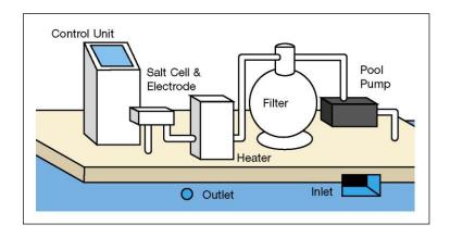
Once the cell is installed, connect the black multi-core cable from the chlorinator control unit to the cell. The blue wire must be connected to the blue terminal. The (multi-core) 4–wire cable wires are color coded to match their corresponding connection points in the cell—the posts fit into the corresponding color keyed sockets on the connector end of the cell housing. The cable is designed to come from below the cell. Make sure wing nuts are correctly tightened to ensure good contact.
