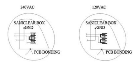
At the bottom of the Salt chlorinator there is a connection that should be used to ground the unit to the pool grounding system with a copper wire of 8 AWG (6 AWG for Canada) (as per diagram below)
