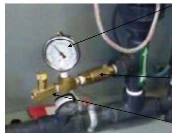
Sonoxides shipped after 8/09 will be equipped with this vacuum valve and gauge assembly
