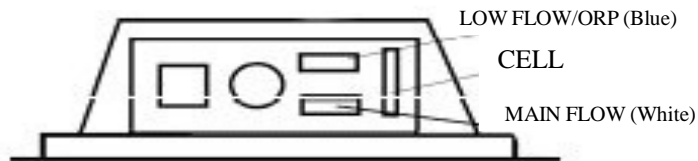
BOTTOM PANEL OF THE MINERAL SPRINGS UNIT
